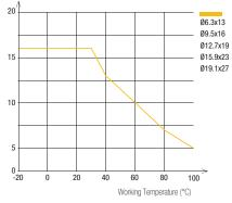
To calculate burst pressure, the values in this graph should be multiplied by 3.
