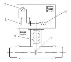
The motion is transferred positively from the baffle (1) to the measuring section.
