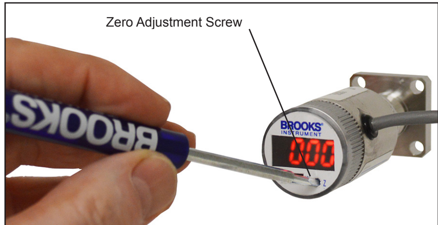
Figure 2-9 Location of the Zero Adjustment Screw on the Integrated Display SolidSense II Pressure Transmitters
