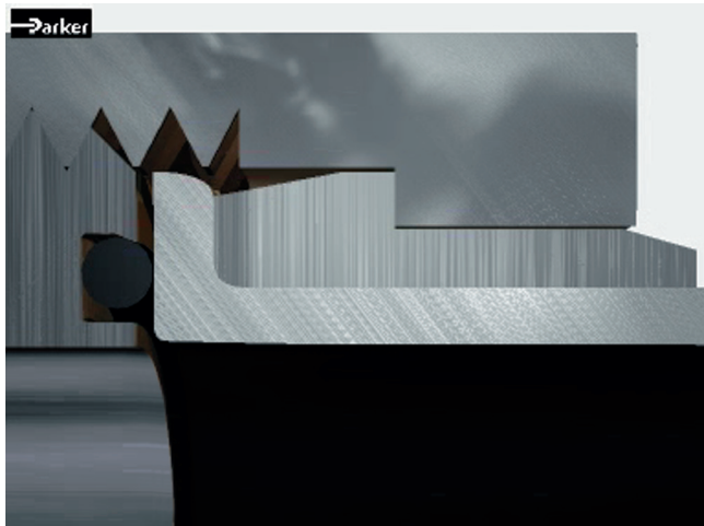
Before tightening the nut
