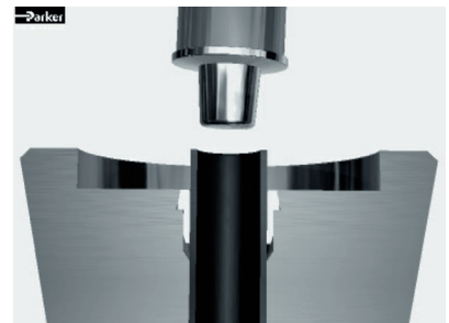
After starting the process, the dies clamp the tube and the flanging pin starts the orbital movement and the forward stroke
