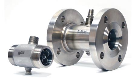
BARTON<sup>®</sup> Model 7400 Precision Turbine Flow Meters are designed for gas service in a wide range of industrial, commercial, pipeline and aerospace applications. Because the output from the pickup coil is digital, Model 7400 meters are an excellent match for electronic output devices — no analog to digital conversion is required. The rotor response is in milliseconds, providing precise metering in applications with rapidly changing flow patterns.
