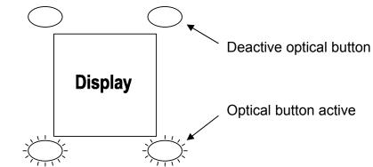
An optical button is located at each corner of the TFT display. The operability of the respective buttons is signaled by blue backlighting; therefore non-backlit buttons are disabled and cannot be operated. To operate the keys, the finger must be placed on the key-dome and raised again. The orange background of the button symbols is briefly displayed in blue as visual feedback for a detected key press.
