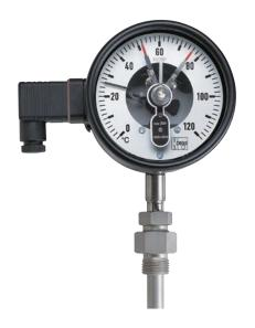
A glycerine filled indicator version is available as an option for service at measuring points exposed to strong vibrations. The fill dampens the measuring system when exposed to mechanical vibrations and thus enables steady indication; it also provides good lubrication for moving parts.
