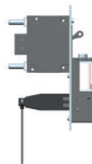
RBR back to initial configuration (by gravity)
