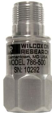
Wilcoxon's intrinsically safe 786-500-IS sensor is certified for usage in hazardous areas and offers clear signals at low vibration levels. The sensor is designed with extended low-end frequency response and improved signal-to-noise ratio compared to other general purpose models. It can be used to detect both low- and high-speed vibrations and is optimized for detecting vibration on slow turning machinery such as cooling tower fans and slow-speed gearboxes.
