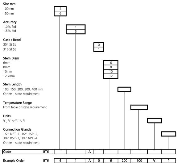
Any Angle Bi-metallic Thermometer, 100mm Dial, 1% Accuracy, 304 St St Case, 6mm stem, stem length = 200mm, range 0-100 Deg C, 1/2" NPT connection
