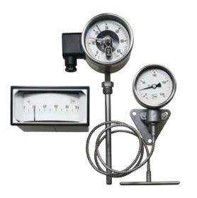
A version filled with glycerine is available as an option for service at measuring points exposed to strong vibrations. The fill dampens the measuring system when exposed to mechanical vibrations and thus enables steady indication; it also provides good lubrication for moving parts.
