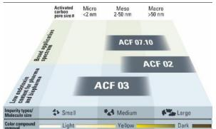
The activated carbon of the BECO CARBON depth filter sheets is a microporous, inert material with a very large inner surface of up to 2000 m<sup>2</sup>/g of activated carbon. The activated carbon used can be divided into different porosity ranges:
