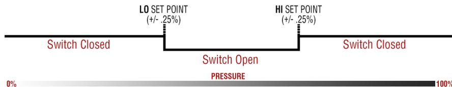
In this configuration, the switch output will be open when the process pressure is within a user selectable range and closed when the pressure is outside of these boundaries. This is designed for applications where there is a known acceptable operating pressure range.
