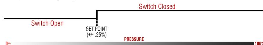
In this configuration, the switch output will be open for pressures less than the selected setpoint. The switch output would then be closed for pressures greater than the setpoint.
