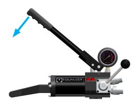
4. Steps 2 & 3 are repeated, which will pump oil into the system until the maximum pressure of 10,000 psi (700 bar) is achieved, at which point the safety release valve will open and the oil will cycle back to the reservoir.
