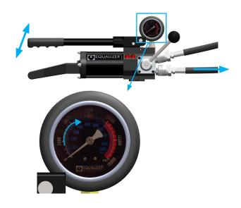
**5.** To depressurise the advance hose move the control lever to the retract position this will redirect the flow to the retract hose.
