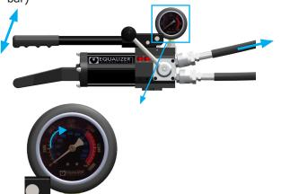
**7.** To keep pressure in both hoses, set the control lever in the central vertical position.
