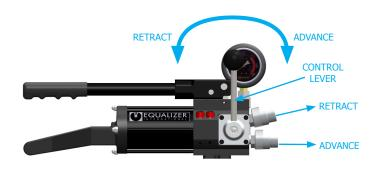
**4.** Pressurise the advance hose by raising and depressing the pump handle until the desired pressure is indicated on the pressure gauge N.B. max. pressure 10,000 psi (700 bar)
