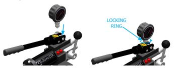
2. Ensure the hydraulic system you wish to pressurise has been bled and is free from air and leaks. Connect the pump into the system using the screw connector supplied with the pump, push the male and female connectors together fully and rotate the locking ring clockwise until fully tight.
