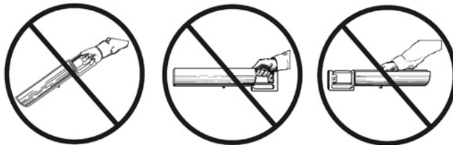
Figure 4-2 Improper handling may functionally destroy the load cell
