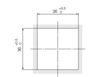
The applicable panel thickness is 1 up to 3,2 mm
