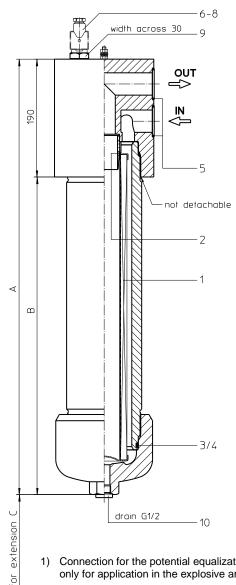
Connection for the potential equalization, only for application in the explosive area.
