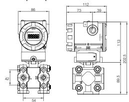
PAD with multi planar flange and angle type bracket\*
