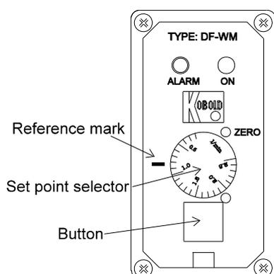
The instrument is delivered ready to operate. The electronics are matched and calibrated with the signal transmitter. The calibration screws ('ZERO' and 'RANGE') next to the rotating scale adjustment knob must not be adjusted by the customer. If they are adjusted, a re-calibration will be required involving new calculations. Should the electronics be opened, any warranty will become invalid.
