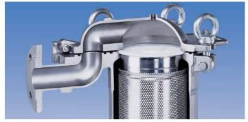
Top inlet connection with hinged cover make filter bag change-outs quick and easy Picture reference to flow design, identical to standard bolted Topline.
