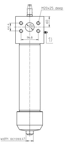
1) Connection for the potential equalization, only for application in the explosive area.
