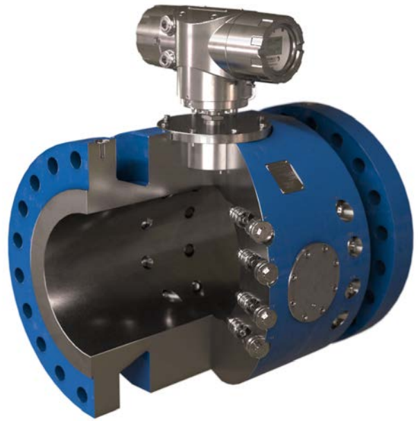
Eight-path chordal design that ensures accurate measurements without additional flow conditioners, even in flows containing swirl and asymmetry.
