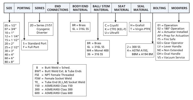
If ball and stem are different materials, expand code to show ball first, stem second. For additional ordering information, see the TBV General Brochure, Corrosion Resistant and Cryogenic Valves.
