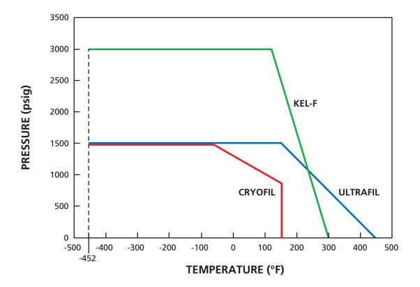
Extended pressures and temperatures may be achieved by altering design for specific applications. Consult factory with service conditions.
