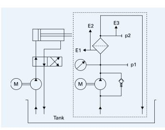
During off-line filtration, the filter operates in a cycle that is separate from the main system. By separating the systems, off-line filtration can take place independently of the system's running time until the desired fluid cleanliness is reached.
