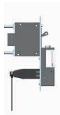
RBR returns to initial configuration (by gravity)
