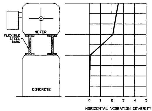
Fig. 11. Plot of vibration (in mils) versus base/motor position.
