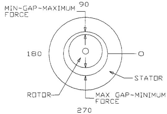
Fig. 4. Unsymmetrical air gap around rotor.
