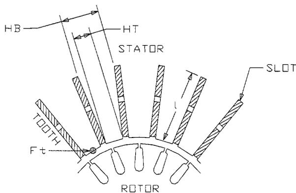
Fig. 10. Stator tooth forces.
