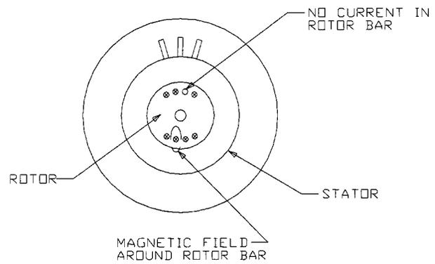
Fig. 6. Rotor with broken rotor bar.
