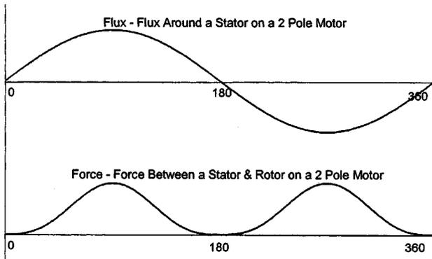
Fig. 2. One period flux wave and magnetic force wave.
