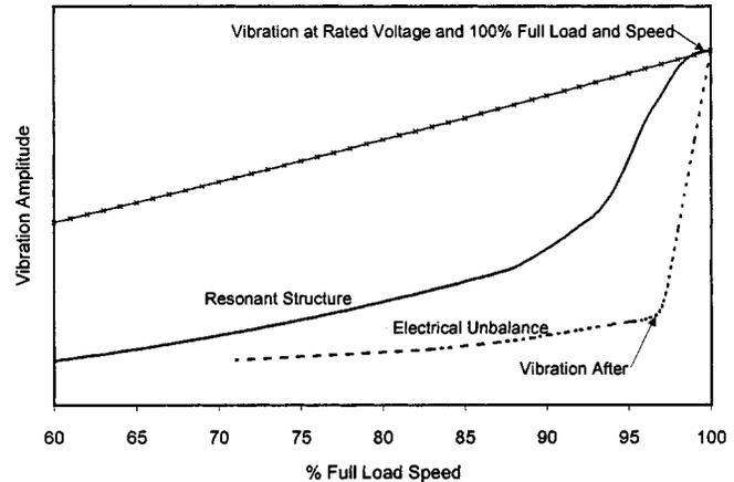
Fig. 16. Vibration after power is removed.
