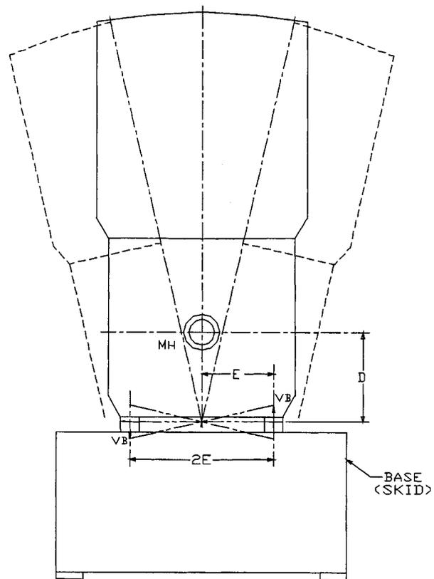
Fig. 12. Rocking mode due to weak base.
