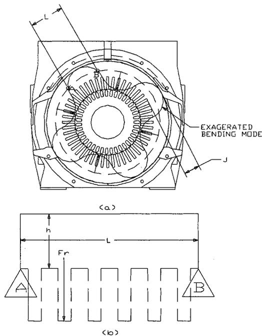
Fig. 9. (a) Fourth mode of vibration. (b) Linear representation of core for one-half wavelength of force.
