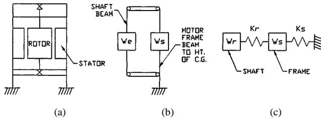
Fig. 13. Structural representation of vertical motor for reed critical frequency calculation including rotor shaft flexibility ( $W_R$ : rotor weight;  $W_S$ : stator weight (motor weight-WR);  $K_R$ : motor shaft and bearing stiffness (lb/in);  $K_S$ : motor frame stiffness (lb/in, considering bending, shear deflection, and flange bending).
