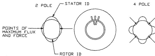
Fig. 3. Electromechanical force on two- and four-pole motors.
