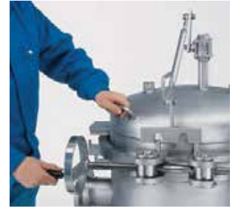
2. Rotate the spindle using the hand wheel to open the V-clamp into the end position.
