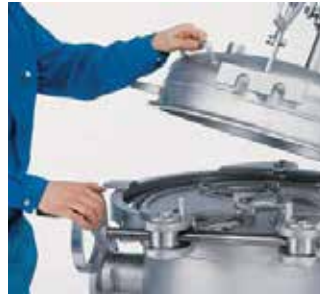
3. Open the cover aided by spring-assisted mechanism.
