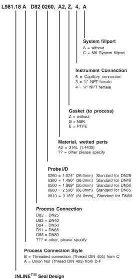
L981.18 = INLINE<sup>™</sup> sanitary diaphragm seal DIN 11851
