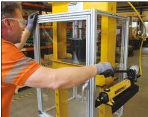
◀ Workshop press with safety cage to ensure additional operator safety.
